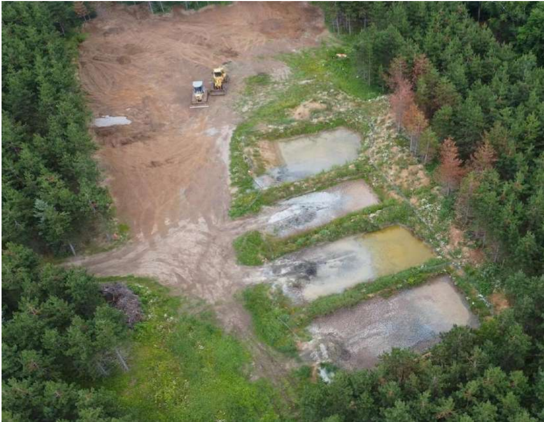
Unlined Sumps: Drill Cutting Waste (Wildflower Group, 2023)
